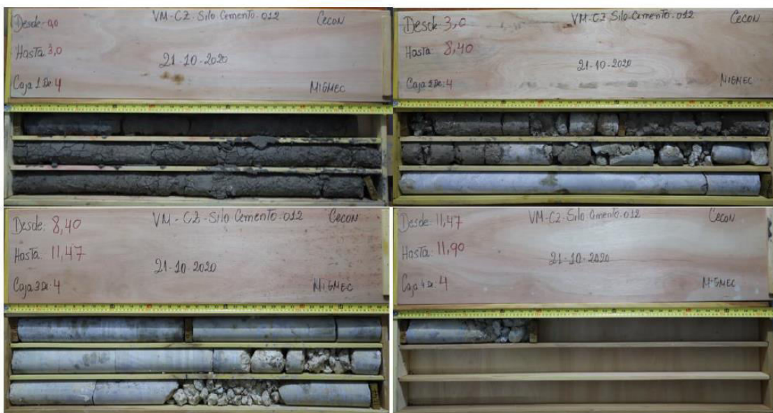
Figure 3. Soil and rock core drilling for borehole VM-CZ (CECON SAE, 2020).
