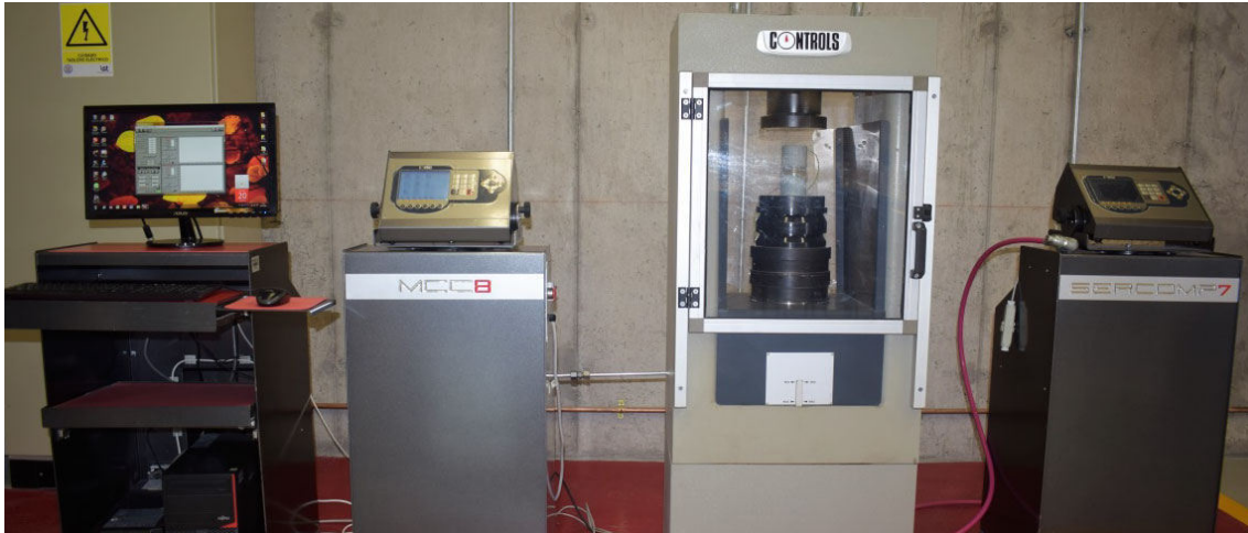
Figure 3. Rock strength testing machine, Controls MCC8 50-8422/M and triaxial module Controls SERCOMP 7 50-C7022/S available on the Rock Mechanics Laboratory of the Department of Metallurgical and Mining Engineering of the Universidad Católica del Norte
