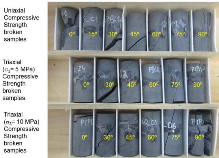
Figure 1. Slate cylindrical specimens cut with different angles in relation to cleavage, showing varied fracturing patterns after compression tests at different confinement levels. Tested at the laboratory of the University of Vigo according to Alejano et al. (2021).
