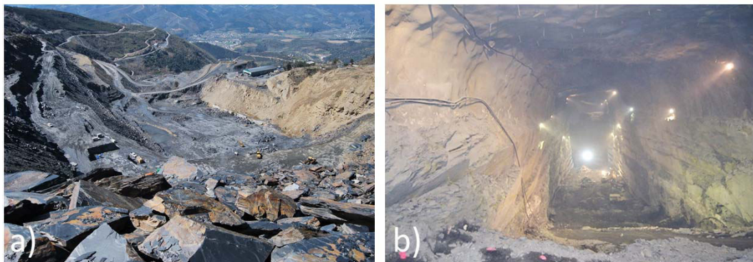
Figure 2. a) Roofing slate quarry and b) Roofing slate underground mine: 25-m wide and 50-m high room.
