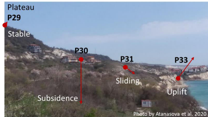
Figure 24. Schematic illustration of estimated displacement directions at selected points.
