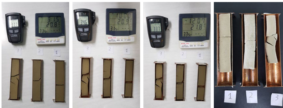
Fig.2. Linear shrinkage limit (LS) test as parameter to identify swelling potential
