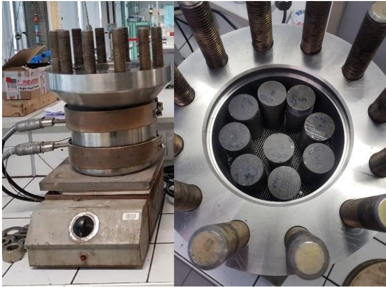
Figure 2: Cell used for subjecting cement samples to CCS conditions
