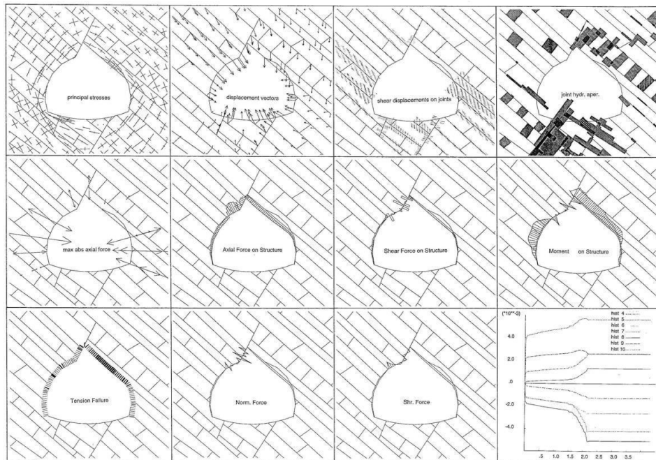
Figure 9. The discontinuum-modelling advantages of representing adversely steeply-dipping bedding. This late 1980's UDEC-BB model of a tunnel in Japan showed distinct signs of over-loading of the bolting. The bonding failure of the modelled S(fr) is also shown, bottom left.
