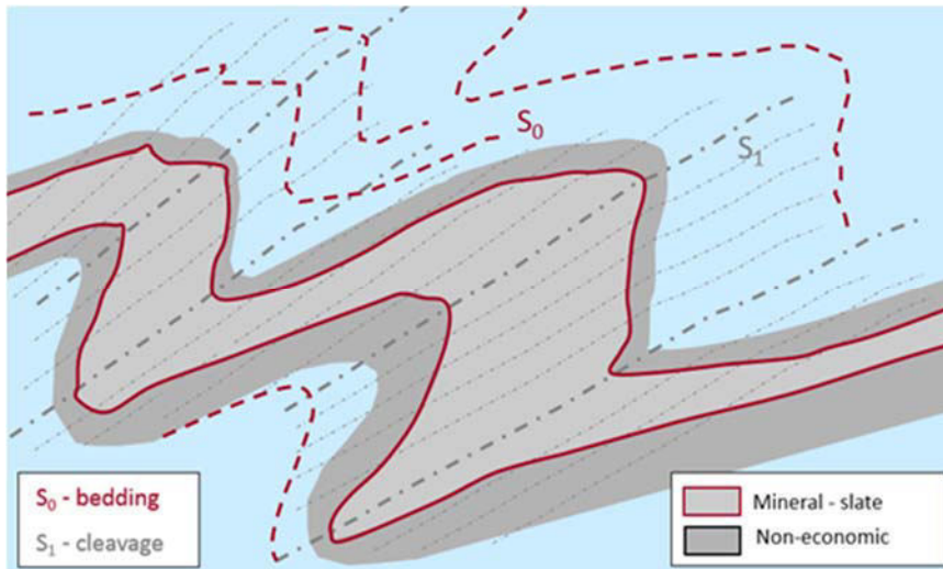
Figure 4. Typical asymmetric fold, whose inverse limb can make out a good roofing slate deposit.
