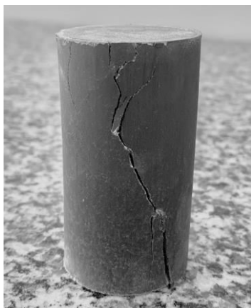
Figure 4. Rock after UCS test, with defined rupture plane.
