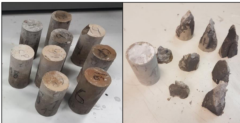
Figure 2. Uniaxial compression test on carbonated samples.
